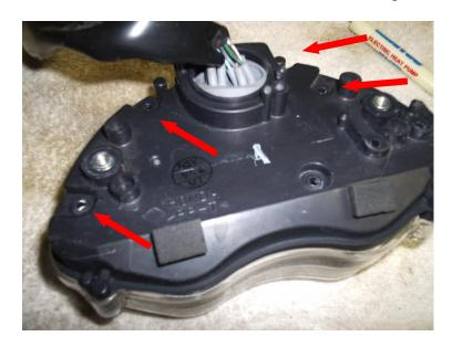
9) Remove four (4) black screws, white washers from speedometer assembly faceplate.
