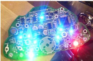
(Sorry, I did not get a good photo of LED's on top side of board. They are small white squares, with corner notched for polarity. You can see by this photo where they are on the board.)
