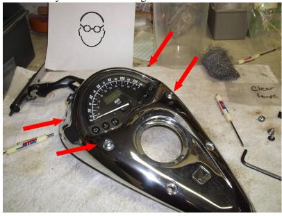
4) Remove two (2) short silver screws – separate speedometer assembly from bracket.
