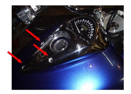
3) Moving to work bench, remove remaining four (4) screws holding speedometer assembly to chrome housing.
