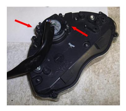
8) Remove four (4) black screws, remove back of speedometer assembly.
